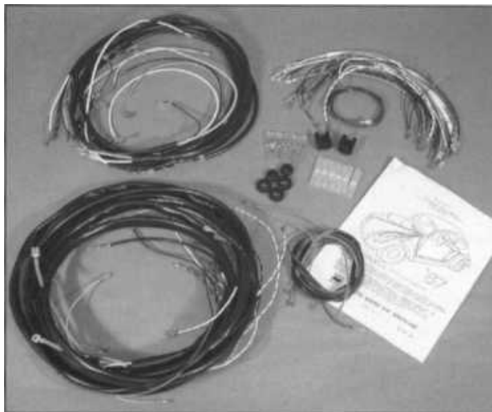
Complete wiring harness for the 1967 VW sedan came from The Real Source, along with new switches, lenses and turn signal lever.
