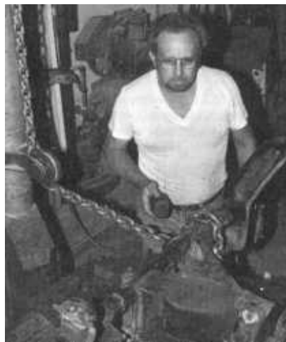
ABOVE, with the rear of the pan chained down, the right front was pulled out until the front-to-rear measurement matched. BELOW, with everything unbolted inside and outside, our pan was sandblasted clean.
