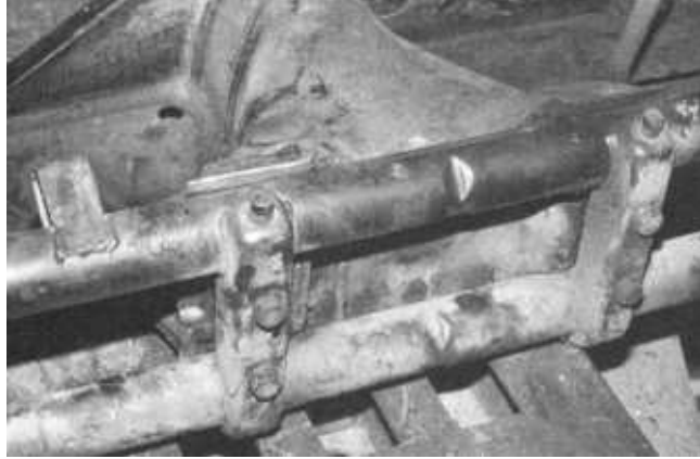
ABOVE LEFT, arrow points to our first problem; a bent front bulkhead. This car was probably crashed hard on the right front, bending the pan. ABOVE RIGHT, after repair, the frame head fit the front torsion tubes squarely.
