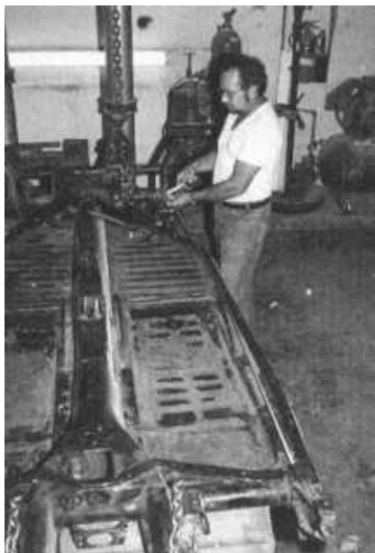
ABOVE LEFT, our pan was placed on Al Martinez's chassis fixture. Measurements showed the right side was bent back almost 3/8-in. For reference, we used the rear corner body fastener holes as a rear measurement point. ABOVE RIGHT, with the right side of the front beam chained to the fixture, heat was applied to the bulkhead.
