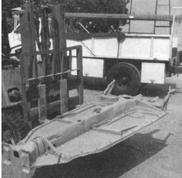
ABOVE LEFT , one hour later, our newly sandblasted pan looks a bunch better for only $35. TOP RIGHT , to gain access to the center clutch tube weld, a small "window" had to be cut into the tunnel. Drill four pilot holes and then use an air chisel (note protective ear and eye wear).
