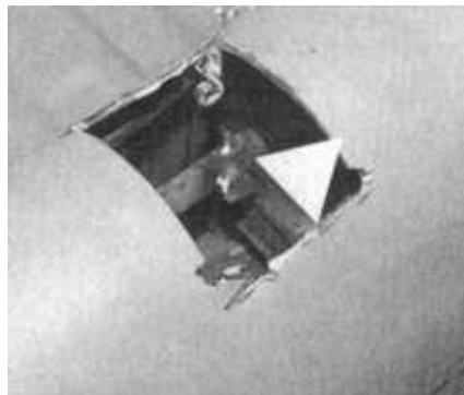
ABOVE , Tim Orchard used a MIG welder to put things back together. Be careful not to distort the tube. BELOW , moving to the front tube mount, a window was cut into the top of the tunnel. Here again, the tube needs to be rewelded back to the bracket.
