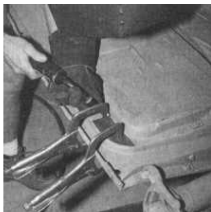
ABOVE , with the tubes fully rewelded back to their brackets, the panels can be welded back into place. Carpeting will cover this later. BELOW , since our pan's rear floor jack brackets were removed, we reinforced the pan with an extra piece of sheet metal.
