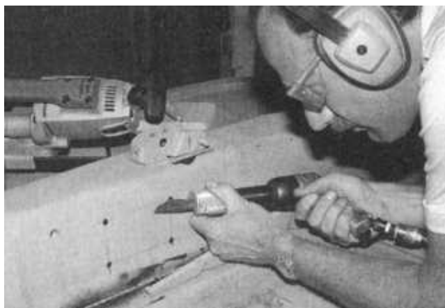
ABOVE LEFT , one hour later, our newly sandblasted pan looks a bunch better for only $35. TOP RIGHT , to gain access to the center clutch tube weld, a small "window" had to be cut into the tunnel. Drill four pilot holes and then use an air chisel (note protective ear and eye wear).
