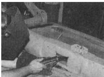
ABOVE , Tim Orchard used a MIG welder to put things back together. Be careful not to distort the tube. BELOW , moving to the front tube mount, a window was cut into the top of the tunnel. Here again, the tube needs to be rewelded back to the bracket.
