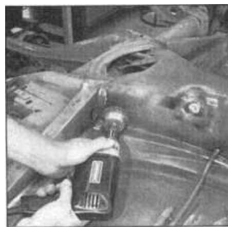
ABOVE LEFT , to remove some of the zillions of dents usually found on a floor pan, Tim Orchard used a hammer and dolly. BELOW , a wire wheel attachment helped remove weld caulking.
