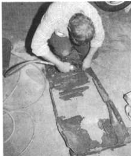
ABOVE , after removing the seats and carpeting, the interior floor pan will be exposed. Pry the outer edge of the pan down from the heater channel, taking care not to damage the pan gasket. Then use an air chisel to break the welds along the tunnel, and front and rear of the floor.
