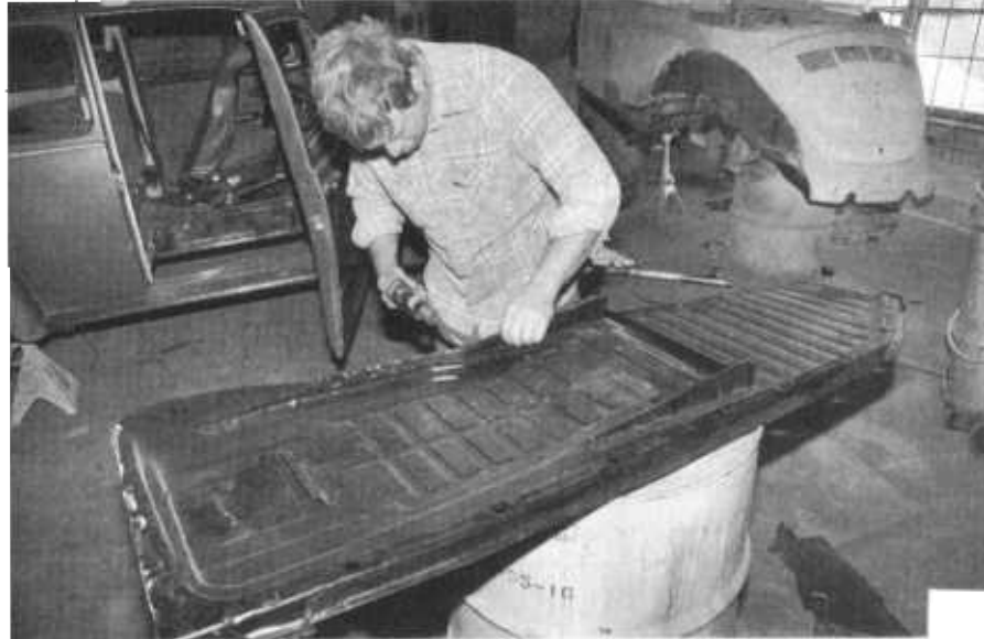
ABOVE LEFT , the first step of our repair required removing the nine body bolts along the outer edge of the floor pan that secure the floor to the body. RIGHT , if you are working on the right side of the car, it is wise to carefully relocate the gas tank evaporator hose. Welding, grinding and gasoline fumes are not a good combination.
