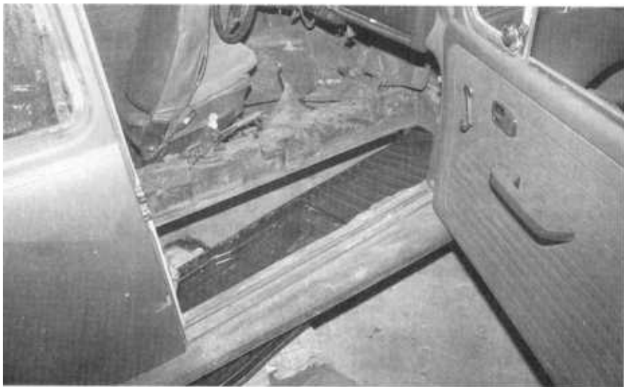
ABOVE , clean and grind off all old welds along the bottom edge of the tunnel where you will be welding to ensure a proper fit. Position the new floor back in the opening after mounting the original pan gasket.
