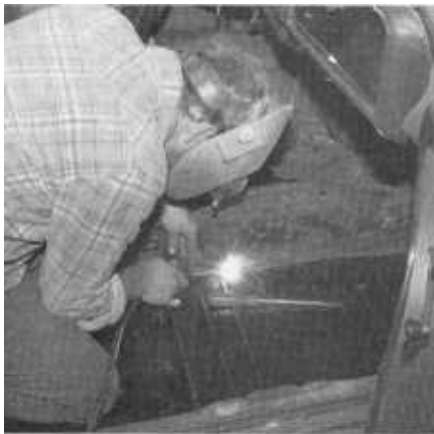
ABOVE LEFT , complete the welding by laying short beads, approximately 1.5-in. long and four inches apart, along tunnel-side of the floor. To prevent warpage, jump around and keep heat buildup to a minimum. Weld front and rear in place using the same method. ABOVE RIGHT , now weld old seat pedestal in place on the new floor panel.
