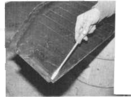
TOP , if using the later seats, remove the rails from the new pan with an air chisel. RIGHT , now carefully remove the seat pedestal from the old floor. ABOVE LEFT , check pedestal fit by placing on the new pan, and trim as necessary to fit — don't weld in place until the pan is in the car. RIGHT , check the new panel for fit, it may be necessary to trim and notch the front edge to clear a factory weld.
