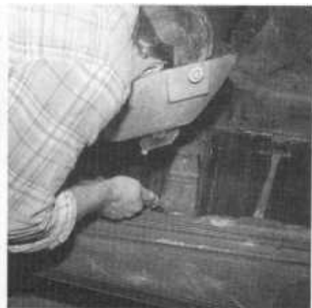
ABOVE LEFT , complete the welding by laying short beads, approximately 1.5-in. long and four inches apart, along tunnel-side of the floor. To prevent warpage, jump around and keep heat buildup to a minimum. Weld front and rear in place using the same method. ABOVE RIGHT , now weld old seat pedestal in place on the new floor panel.
