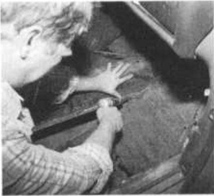
ABOVE , after removing the seats and carpeting, the interior floor pan will be exposed. Pry the outer edge of the pan down from the heater channel, taking care not to damage the pan gasket. Then use an air chisel to break the welds along the tunnel, and front and rear of the floor.
