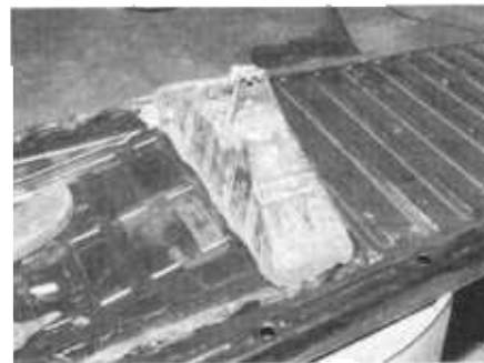
TOP , if using the later seats, remove the rails from the new pan with an air chisel. RIGHT , now carefully remove the seat pedestal from the old floor. ABOVE LEFT , check pedestal fit by placing on the new pan, and trim as necessary to fit — don't weld in place until the pan is in the car. RIGHT , check the new panel for fit, it may be necessary to trim and notch the front edge to clear a factory weld.
