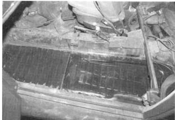
ABOVE LEFT , reinstall the nine bolts then secure the floor to the outer portion of the car making sure the gasket is aligned. ABOVE RIGHT , press the two pieces together on the tunnel-side edge of the floor and tack weld in position. Use a body hammer to knock down any high spots. This is how the section will look once installed.
