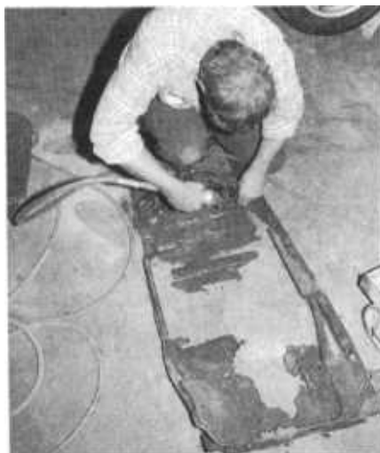
ABOVE , after removing the seats and carpeting, the interior floor pan will be exposed. Pry the outer edge of the pan down from the heater channel, taking care not to damage the pan gasket. Then use an air chisel to break the welds along the tunnel, and front and rear of the floor.
