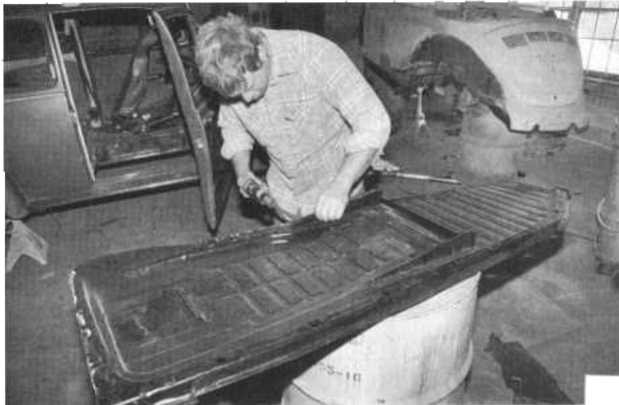
ABOVE LEFT , the first step of our repair required removing the nine body bolts along the outer edge of the floor pan that secure the floor to the body. RIGHT , if you are working on the right side of the car, it is wise to carefully relocate the gas tank evaporator hose. Welding, grinding and gasoline fumes are not a good combination.
