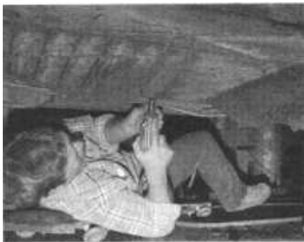
ABOVE LEFT , the first step of our repair required removing the nine body bolts along the outer edge of the floor pan that secure the floor to the body. RIGHT , if you are working on the right side of the car, it is wise to carefully relocate the gas tank evaporator hose. Welding, grinding and gasoline fumes are not a good combination.
