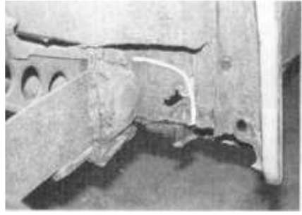
ABOVE LEFT , you can see the backside of the heater channel. ABOVE RIGHT , rocks and road debris chip the coating off the wheelwell and it doesn't take long before the bare metal rusts through at the seam between the heater channel and the fenderwell.
