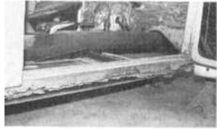
ABOVE LEFT , the replacement heater channel incorporates the upper rocker panel, the front dog-leg extending to the front firewall and the rear connecting pipe. ABOVE , this bottom view shows the fastening panel, or bottom plate. Once installed, this part of the heater channel cannot be seen. BELOW LEFT , remove the interior before starting to avoid damage. BELOW RIGHT , with the running board off (there wasn't anything holding it) you get a good look at an advanced case of heater channel rust.
