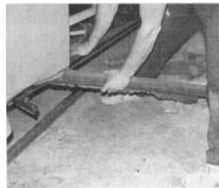
ABOVE LEFT , VW Restorations uses a plasma cutter to remove the old heater channel. Here the channel is being cut along the factory weld at the front door post. CENTER , make another cut at the rear door post along the factory weld seam. Cut right along the weld and clean-up any jagged metal with a die grinder, file, or de-burring tool. ABOVE RIGHT , scrape away the factory seam sealer. RIGHT , the heater channel is also welded to the outer sheetmetal at the bottom of the quarter panel just above the jack support. Cut along the spots welds and the body seam, the heater channel should come loose from the rear of the car.
